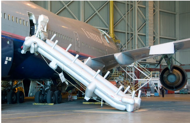
Figure 2.1: Inflated evacuation slide on a B747.
