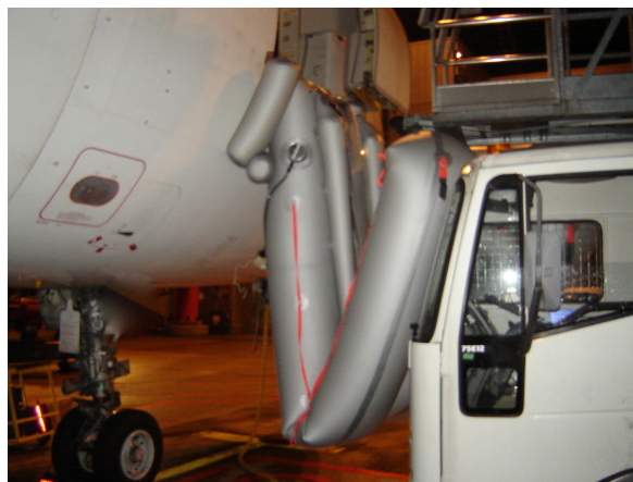
Figure 2.2: Slide deployment event on ground.
