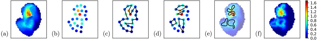
Fig. 2. Steps of our PRO-STM algorithm: (a) input target pressure field, (b) clustering, (c) initial path, (d) split into multiple paths to satisfy length constraints, (e) refinement of the paths to maximize pressure intensity, (f) resulting reconstructed pressure field.
