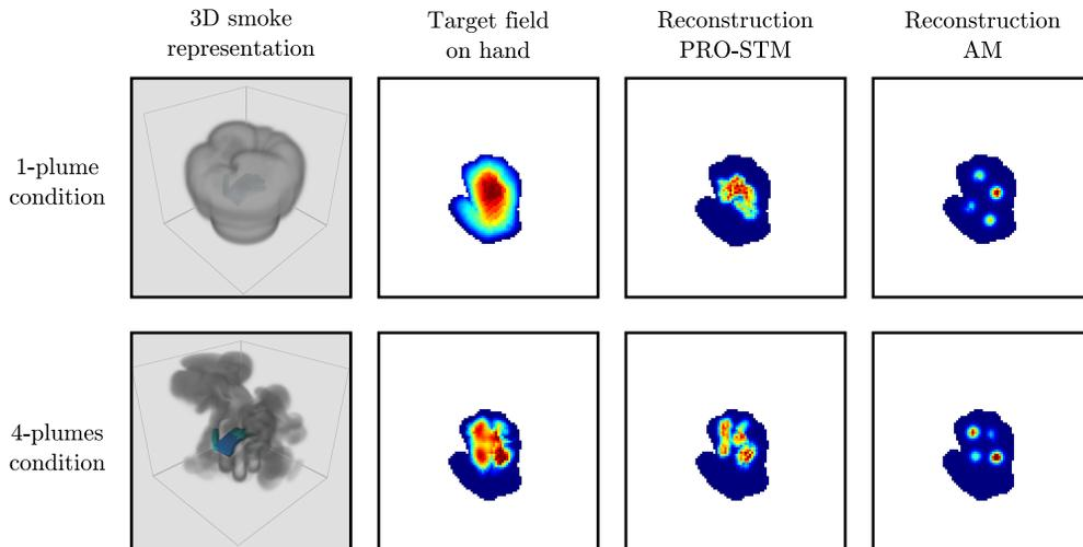
Fig. 3. Experimental scenarios and representative examples of target and reconstructed fields using the proposed method (PRO-STM) and a previous AM method [4].
