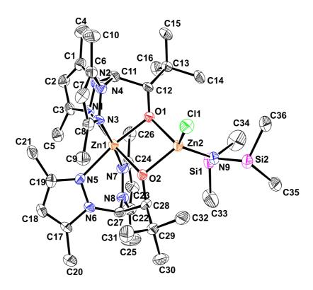
**Figure 3.** ORTEP view of the S,S enantiomer of  $[Zn(bpzbe)_2(ZnCl{N(SiHMe_2)_2})]$  (8). Hydrogen atoms have been omitted for clarity. Thermal ellipsoids are drawn at the 30% probability level.
