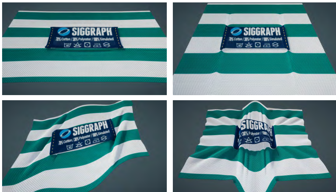
Figure 4.7: Snapshots of simulations of a shirt neck tag. The tag is roughly 5 times stiffer than the shirt, and is stitched on the sides. We apply different deformations to the underlying shirt fabric, from left to right: horizontal stretch, vertical stretch, shear followed by vertical stretch in the middle, and vertical stretch in the middle followed by horizontal compression of the tag. The difference in stiffness induces sliding of the layers, as well as wrinkling at the interface (see first and third snapshots). The last example shows the separation of the tag as it buckles. We trigger the separation of EoL contacts automatically by checking the sign of the normal force.
