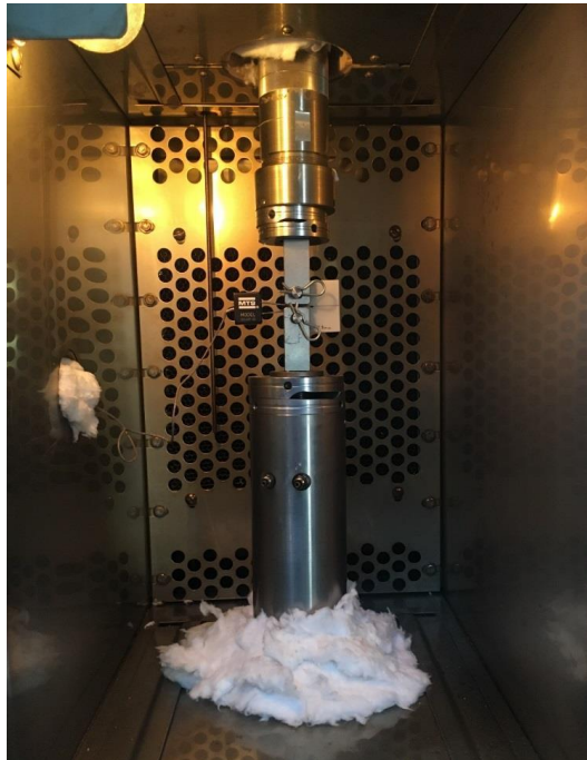
Figure 4-8. Load train assembly inside environmental chamber MTS 651.06E-03 for tests at -50 °C and 50 °C.
