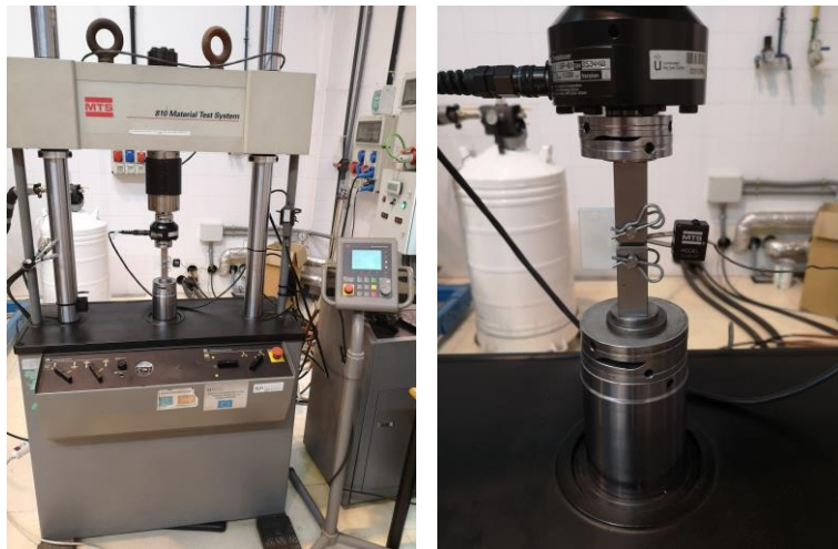
Figure 4-9. MTS 810 Materials Testing machine configured for performing fatigue crack growth tests in CT specimens.
