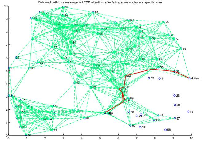
Fig. 3. Illustration showing the path followed by a message generated at node 45 until it is delivered to the sink (node 4) according to *Scenario C* in LPGR. Nodes without a line to their neighbors have used up their batteries or have suffered from failures.
