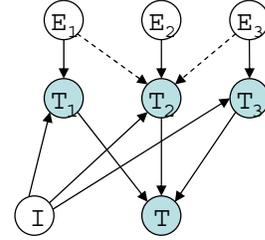
Fig. 2. The graphical model built by a transmitting node including the importance of the message and the energy of the neighboring nodes. Each node makes the simplifying assumption that the neighbor decision will not depend on the energy at other nodes (thus omitting dependencies given by the dashed arrows, that could appear if neighbor are neighbors themselves).
