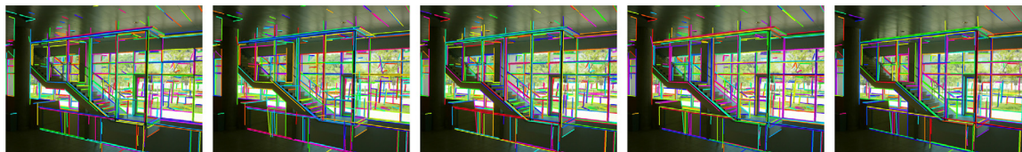
Fig. 11. From left to right: No Validation no jumps, No validation with fixed size jumps (5 px) and no jump validation, No validation with fixed size jumps (5 px) and jump validation, No validation with multi-size jumps (5, 7, 9 px) and jump validation, Validation with multi-size jumps (5, 7, 9 px) and jump validation
