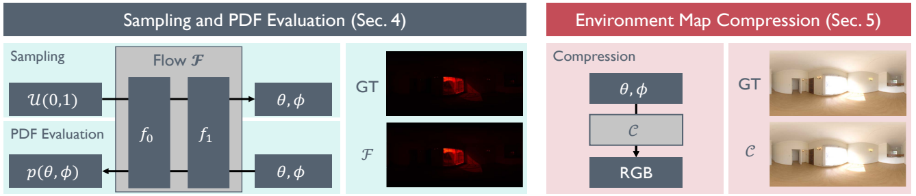
Figure 2: Overview of NEnv. We propose an invertible generative neural network \mathcal{F} (i.e. a normalizing flow) which simultaneously learns to sample directions (\theta, \phi) from an environment map, as well as evaluating the probability of a given direction. This model, illustrated on the left, can be integrated seamlessly into path tracer render engines, allowing for efficient multiple importance sampling. We additionally use a implicit neural representation \mathcal{C} (second column) which learns to map from directions to linear RGB values, allowing for faster evaluation.
