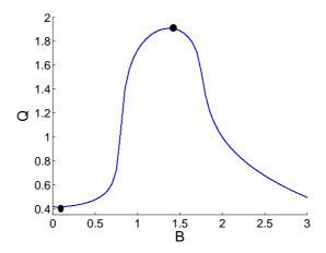
FIG. 1: Typical VR curve, the response of the system Q is plotted vs the amplitude of the HF signal B. The parameters of equations (3-4) are chosen to be  $\alpha = 2.5$ ,  $\beta = 2$ ,  $\tau = 0.5$ , A = 0.1,  $\omega = 0.1$  and  $\Omega = 5$ . These will be the standard parameters along this work if not specified.
