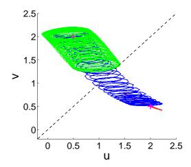
FIG. 2: Phase diagram. The dashed line represents the separatrix (u = v) and the magenta crosses are the two equilibria states  $(e_1 = (0.5, 2), e_2 = (2, 0.5))$ . In red B = 0.1, only one region below the separatrix is explored; in blue B = 1.5, both regions are explored making the amplitude higher (VR); in green B = 2.2, only the region above the separatrix is explored.
