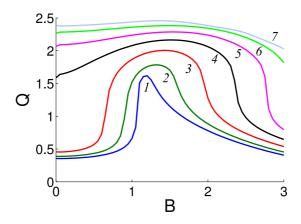
FIG. 8: Effect of the variation of the delay  $\tau$  in the response of the system, when  $\tau < 1$ . For the curves 1-7,  $\tau = 0.35, 0.45, 0.55, 0.65, 0.75, 0.85, 0.95$ . For  $\tau > 1$  autonomous oscillations occur.
