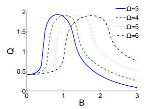
FIG. 6: In this plot  $\Omega$  is varied keeping the other parameters constant. The VR curve presents a shift in the amplitude of the HF signal B at which resonance occurs. However, the maximum value of Q is barely changed.
