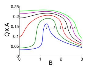
FIG. 4: Resonance curves for different amplitudes of the LF periodic signal  $A=0.09,\ 0.1,\ 0.11,\ 0.12,\ 0.13,\ 0.14$  (curves 1-6 respectively). Notice that in this case Q is multiplied by A for clarity of the plot, otherwise the curves would cross. The shape of the curves remains unaltered, so we can appreciate the widen of the peaks. Above some threshold ( $A\gtrsim 0.15$ ) resonance without tuning occurs.
