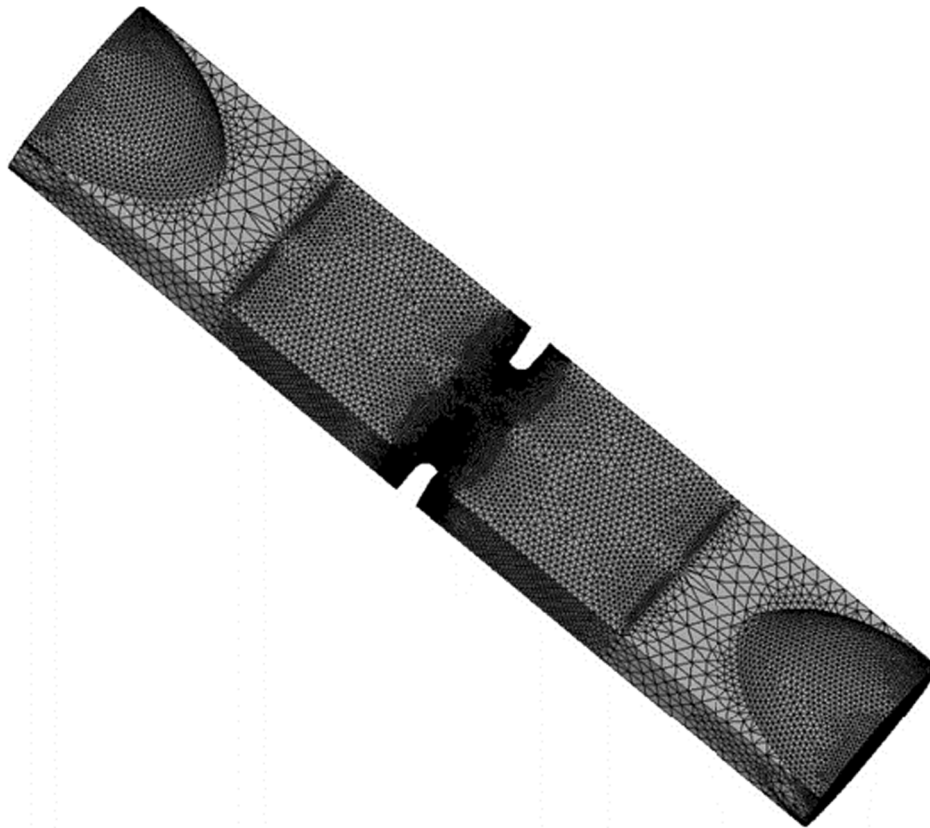
Fig. 6. Full geometry and mesh of the specimens (notch tip radius of 0,5 mm) used in ANSYS and LS-Dyna. Only one quarter was modelled due to symmetry.
