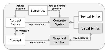
Figure 1. Syntaxes and Semantics of a DSL (adapted from [11])
