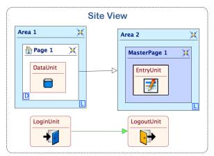
Figure 5. Main composition rules of WebML Visual Notation
