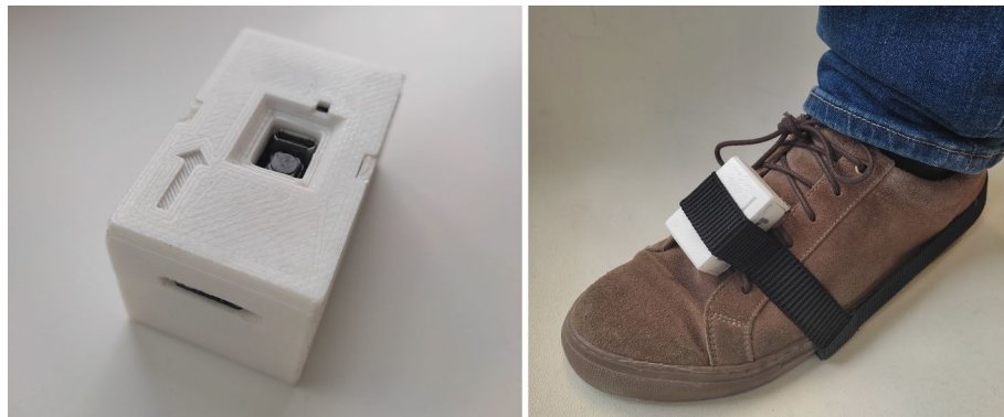
Figure 1. G-STRIDE IMU. Left: unit for tests. Right: IMU attached to a participant's foot.
