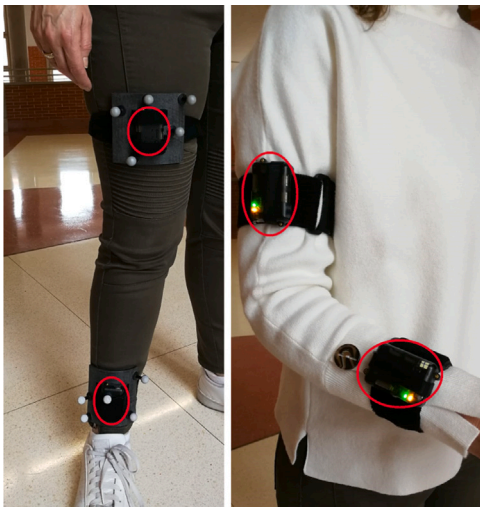
Fig. 2. IMUs placed at the right lower-limb and at the right upper-limb, marked with red circles. On the left limbs, there are two more IMUs at similar placements than in the right upper-and lower-limbs, respectively. Passive reflector sensors, which are commonly used to obtain optical reference data in biomechanical studies as in García-de-Villa, Jiménez-Martín, and García-Domínguez (2021) , are also shown. However, the optical data are not used in this study.
