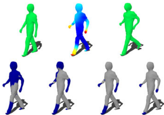
Figure 4. Top row: left and right, two equivalent poses of walk and run sequences. In the middle, the resulting linear blended mesh, coloured using a heat-map (red largest error) to display the errors with respect to the non-linear result. Bottom row: results of our hybrid approach using different threshold \epsilon (3, 6, 8 and 14 mm.). Grey represent areas with errors below the threshold (non corrected), and blue represents areas above the threshold that have been corrected.
