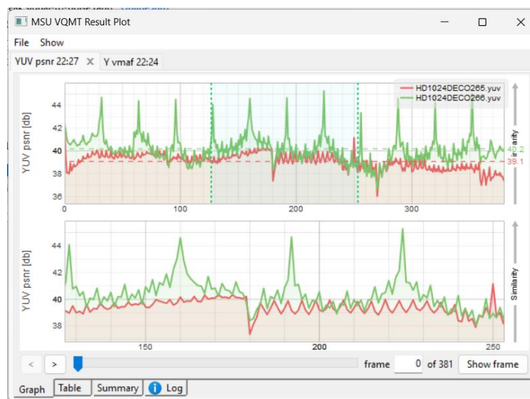
Figura 11. Cálculo PSNR en MSU Video Quality Measurement Tool
