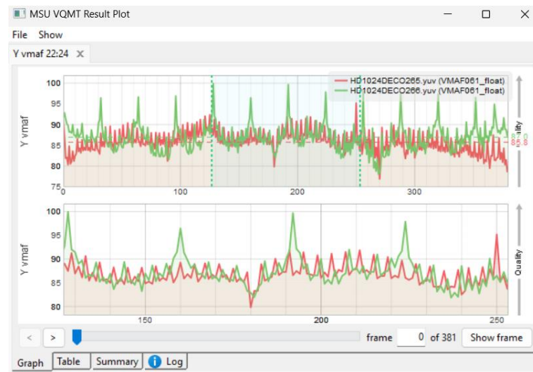
Figura 15. Cálculo VMAF en MSU Video Quality Measurement Tool
