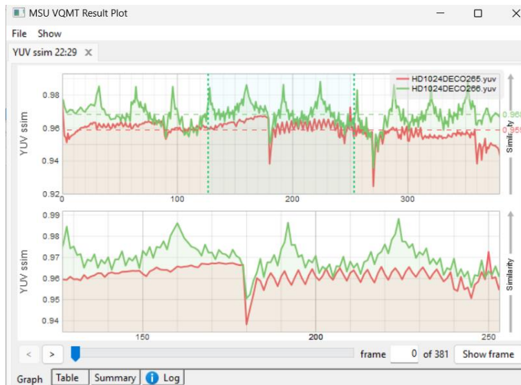
Figura 19. Cálculo SSIM en MSU Video Quality Measurement Tool
