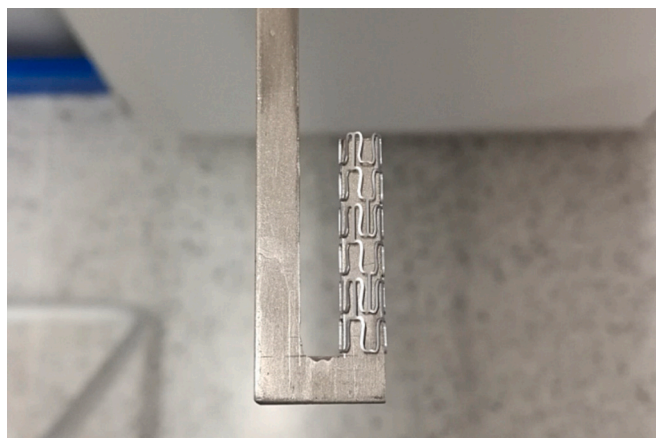
Fig. 4. Stent inserted on a titanium hook prior to the PEO process.
