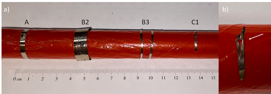
Fig. 2. a) Adaptability tests of A, B2, B3 and C1. b) Detail of the crack in sample C1. The pipe has a 20 mm radius.
