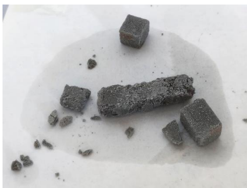
Fig. 54. Propellant material subjected to ozone ageing for a 3-month period.
