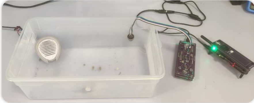
Fig. 95. Ozone ageing chamber with ozoniser and ozone monitoring system.
