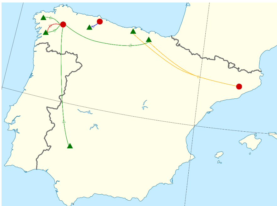
Figure III.26. Collection sites and fractionation plants network for: a) min_CO scenario (blue line), b) min_EQ scenario (yellow line), c) min_HH scenario (green line), d) min_NR scenario (red line). Red dots represent the fractionation plants in each scenario, and green triangles stand for biomass collection sites.
