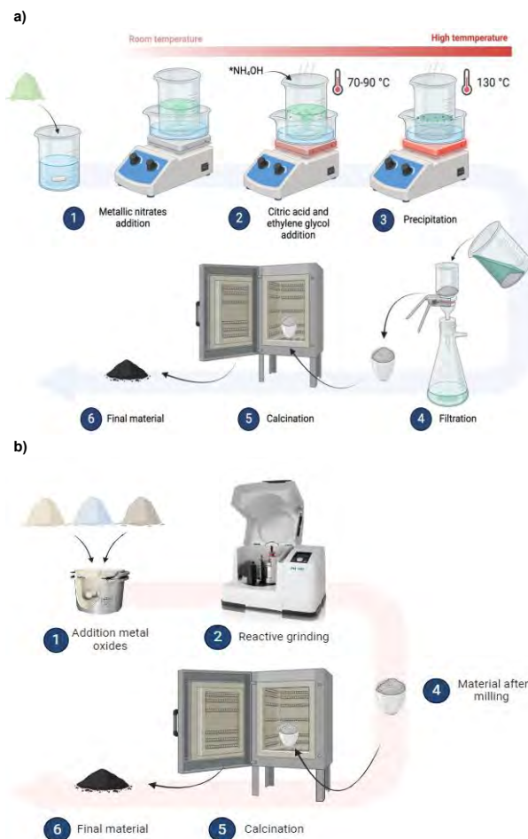
Figure ii. Scheme of the synthesis methods evaluated in this Doctoral Thesis: a) Sol-gel (Pechini) and b) Reactive grinding.
