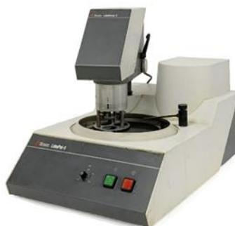
*Figura 3.2. Pulidora Struers Labopol-5*
