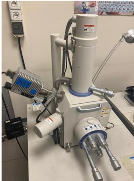
*Figura 3.11. S-3400 N Scanning Electron Microscope.*
