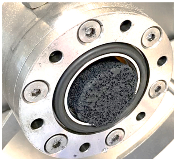
Fig. 2. Picture of the perovskite-based RPC structure inside the high temperature tubular furnace.
