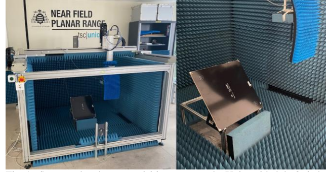
Fig. 16 Setup at the planar acquisition range at the Universidad de Oviedo to evaluate the coverage generated by the SES panel manufactured by Metawave Corp. in Ka-band.
