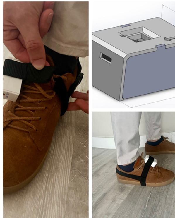
Figure 1. G-STRIDE device attached to a participant's foot.
