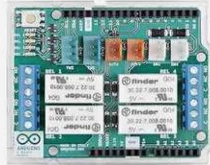
Arduino 4 Relays Shield
