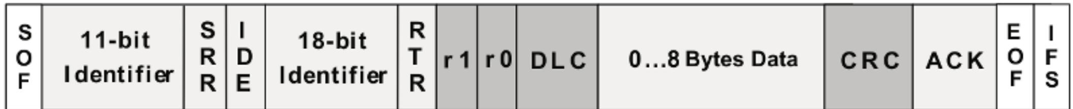
Figure 4. Extended CAN: 29-Bit Identifier
