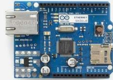
Arduino Ethernet Shield Rev2
