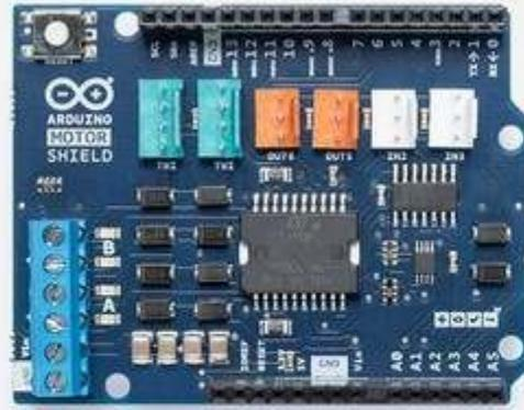
Arduino Motor Shield Rev3
