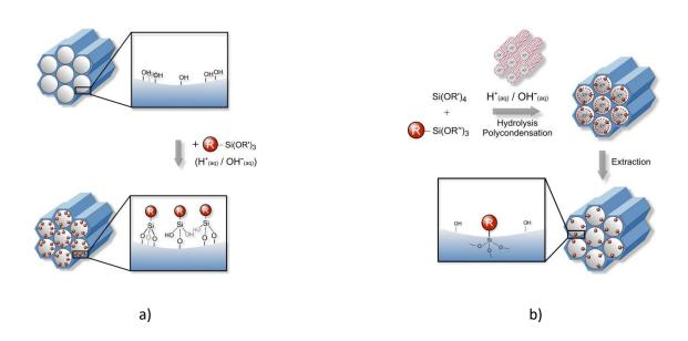
**Fig. 3.** Synthesis of periodic mesoporous silicas (PMOs) from bridged organosilane precursors {Reprinted with permission from [32]}.
