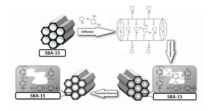
**Fig. 9.** (a) Scheme for synthesis of imprinted mesoporous silica polymer (b) Static adsorption curves of BPA on MIP-MCM-41, NIP-MCM-41, MCM-41, MIP-SBA-15, NIP-SBA-15 and SBA-15 materials {Reprinted with permission from [55]}.
