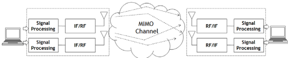
Fig. 11. General architecture of the MIMO measurement system for DVB-T2
