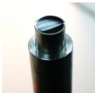
Figure 5. Polished IOFB containing approximately 50,000 fibers.
