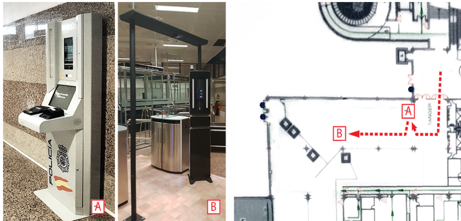
Figure 5: Real scenario with the deployed e-kiosk and e-gate devices.
