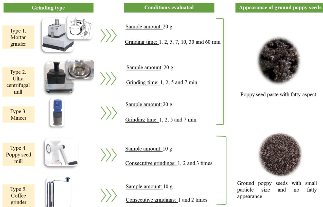
Fig. 1. Types of grindings evaluated with the grinding conditions studied in each of the types (amount of sample and times or consecutive grindings) and the appearance of the ground poppy seed sample.
